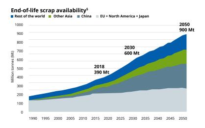
Every steel plant is also a recycling plant, and all steel production uses scrap, up to 100% in the electric arc furnace (EAF) and up to 30% in the blast furnace (BF) route. All scrap that is collected is recycled, and the overall recycling rate today is estimated to be about 85%. This high level of recycling means that there is limited room for improvement.
