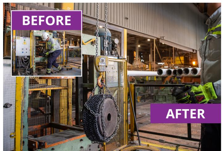
Manual brush exit, starting from the lifting of the object by the operator. ➤ Lifting and transportation of the brush adjusted with hoist transportation.
