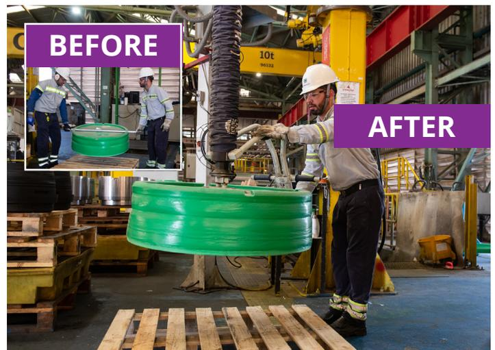
Manual transportation with lifting by two operators. ➤ Hoist-assisted transportation with suction system.
