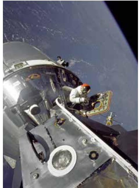
Heat-resistant, 0.0021072 mm thick nickel-steel alloy protected Apollo 9's lunar module from the sun
