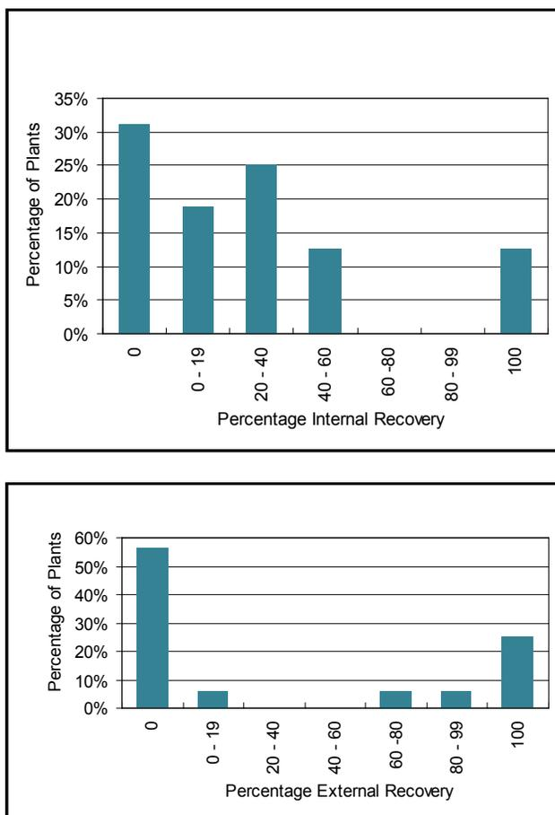
Figure 34 (a) and (b): Distribution of internal and external recovery for BOF SM slag (in %)
