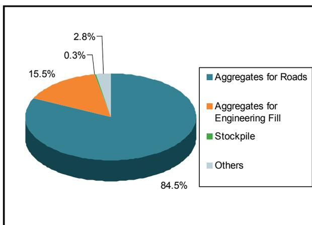
Figure 10: Internal recovery of BF slag as aggregates
