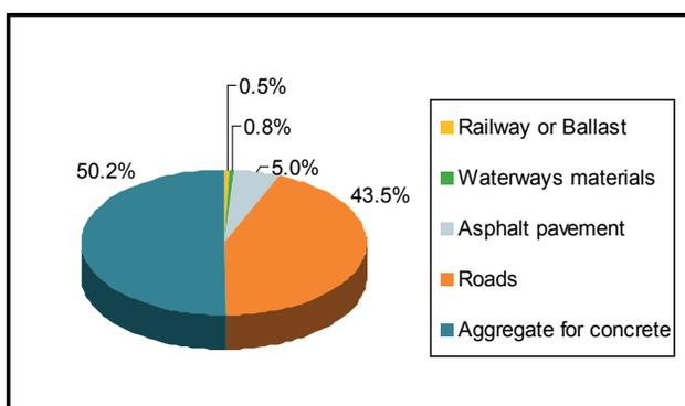
Figure 9: External recovery destinations of BF slag in construction
