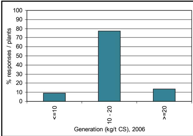
Figure 69: Specific generation of BOF secondary/fine dust and sludge
