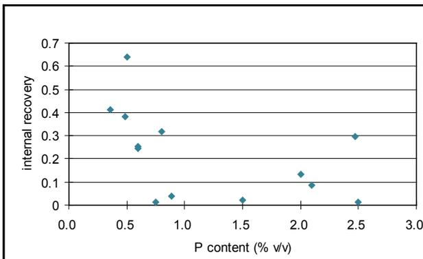
Figure 17: Influence of phosphorus content on the internal recovery in the process
