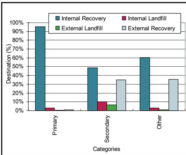
Figure 63: Comparison of BF primary, secondary and other dust and sludge recovery
