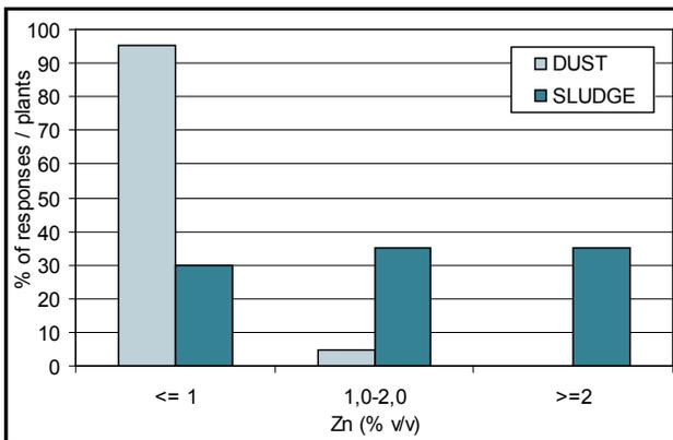
Figure 59: BF top gas cleaning primary and secondary dust and sludge Zn content
