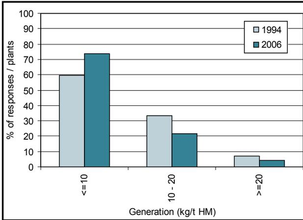
Figure 57: BF top gas secondary dust and sludge generation
