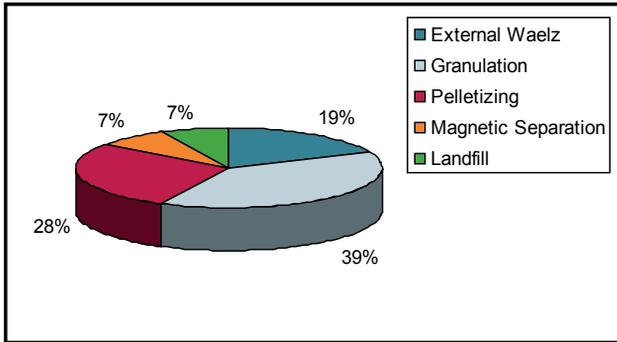
Figure 80: Basic treatments for 'Other' EAF dust and sludge
