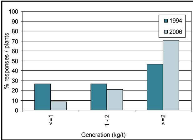
Figure 85: Specific sludge generation in 1994 and 2006
