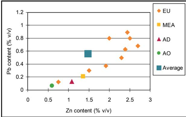
Figure 62: Pb/Zn correlation for BF secondary dust and sludge
