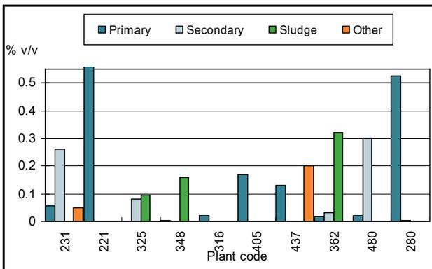
Figure 53: Lead content by plant
