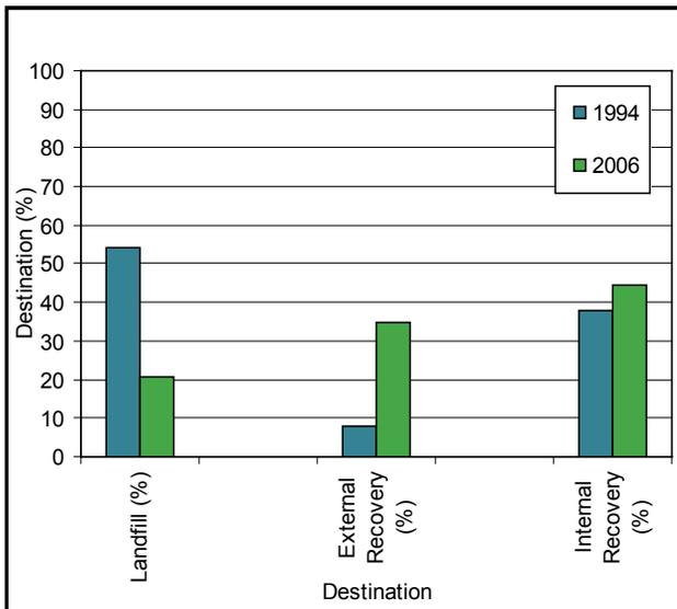
Figure 65: Comparison of BF secondary dust and sludge utilisation in 2006 with 1994 study
