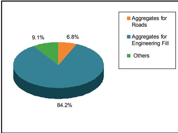
Figure 27: Internal recovery of BOF converter slag in other than process destinations
