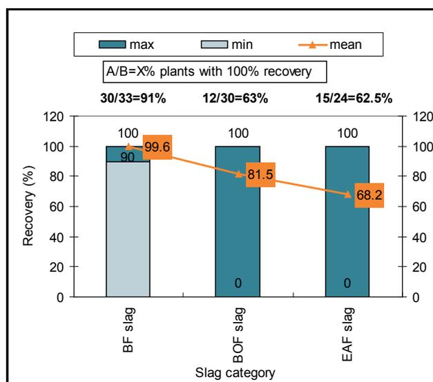
Figure 6: Recovery (external+internal) of slag by category for BF, BOF and EAF slags
