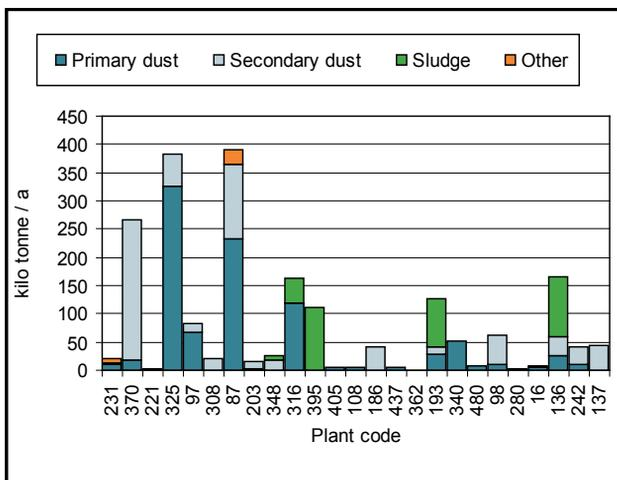
Figure 49: Dust and sludge generation (t/a) in sintering process by facilities
