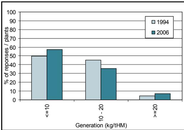
Figure 56: BF top gas primary dust and sludge generation
