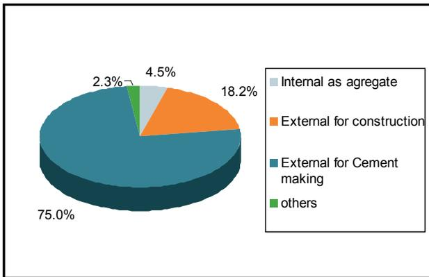
Figure 8: Destination for BF Slag by application
