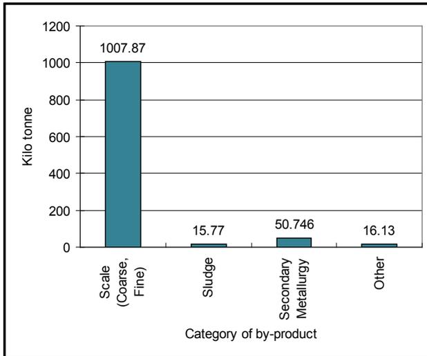
Figure 81: Continuous casting by-product generation (kt)
