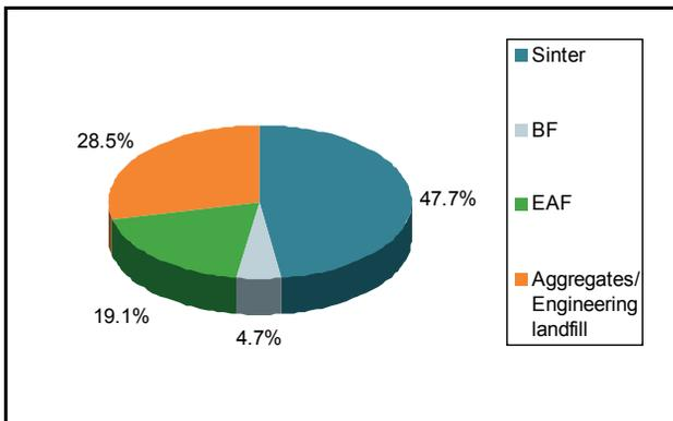
Figure 39: Internal recovery of de-S slag
