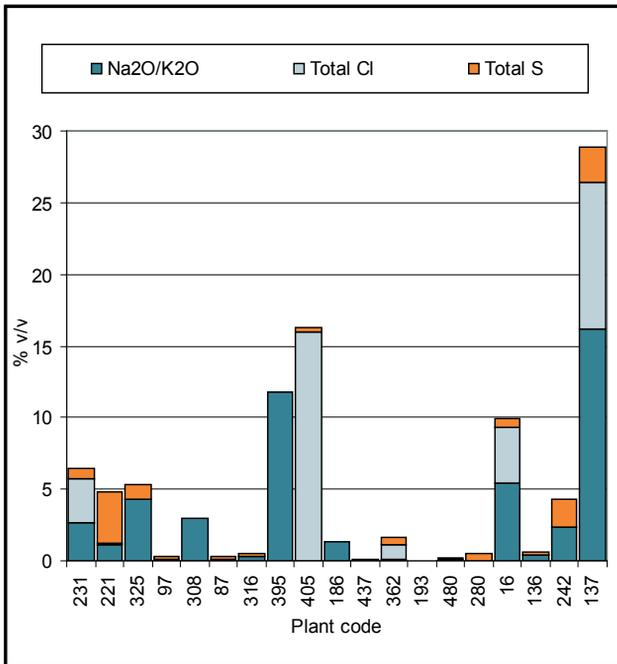
Figure 51: Total Sulphur (S), Total Chloride (Cl) and Sodium/Potassium Oxide ( $\text{Na}_2\text{O}/\text{K}_2\text{O}$ ) content for primary dust and sludge by plant
