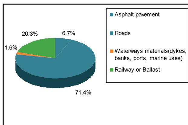
Figure 25: External recovery in construction for BOF slags
