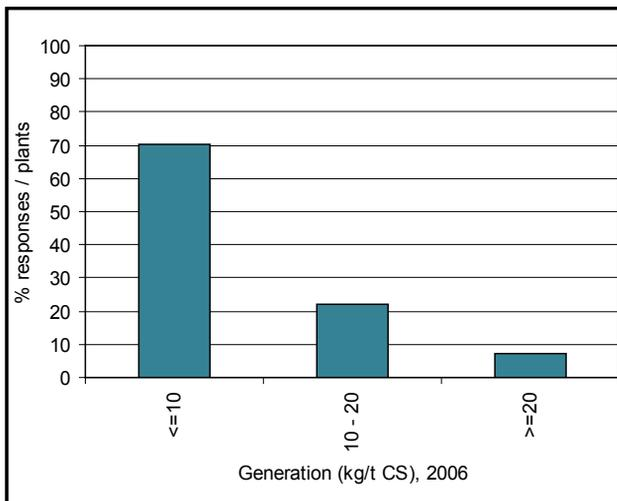
Figure 68: Specific generation of BOF primary/coarse dust and sludge
