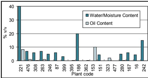
Figure 82: Scale (coarse, fine) moisture and oil content by plant
