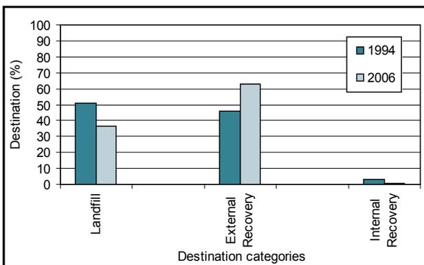
Figure 79: EAF primary dust and sludge utilisation comparison with 1994 data
