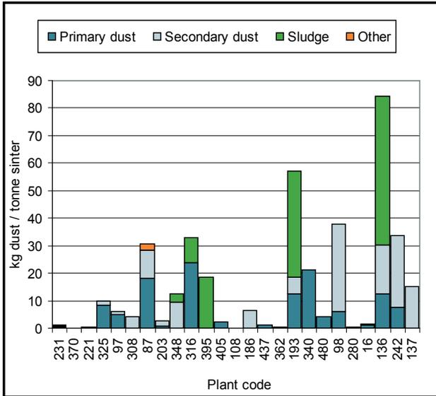
Figure 50: Specific dust and sludge generation (kg dust and sludge/t sinter) in sintering process by facilities
