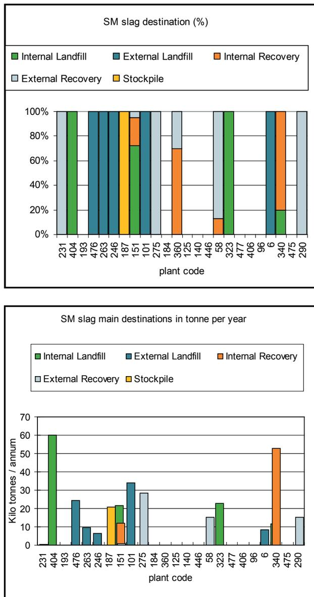
Figure 46 (a) and (b): EAF SM slag main destinations by plant (% and tonnage of generated slag)
