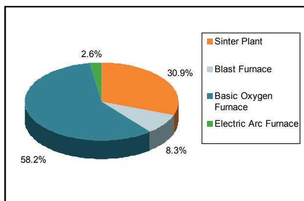
Figure 26: Internal recovery BOF converter slag by process
