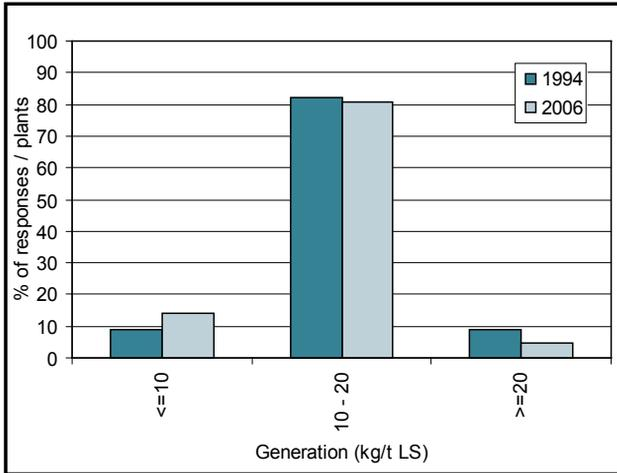
Figure 75: Generation of primary dust and sludge by EAF, comparison to 1994 study
