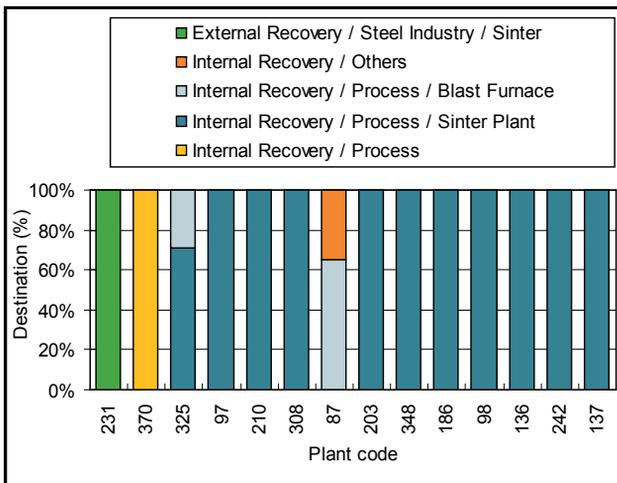
Figure 55: Sinter plant secondary dust recovery rate
