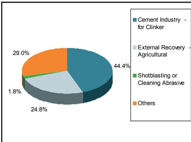
Figure 28: External recovery of BOF converter slag – Other destinations
