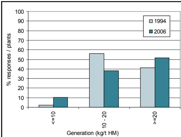
Figure 70: Specific generation of BOF primary and secondary dust and sludge
