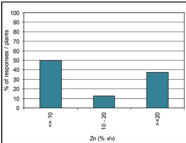
Figure 77: EAF primary dust and sludge zinc content, 2006
