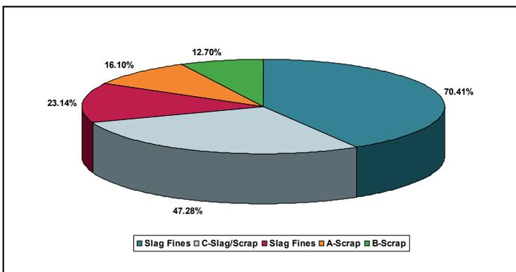
U.S. Steel Figure 1: Product yield from BOP steelmaking in wet kg per ton of liquid steel
