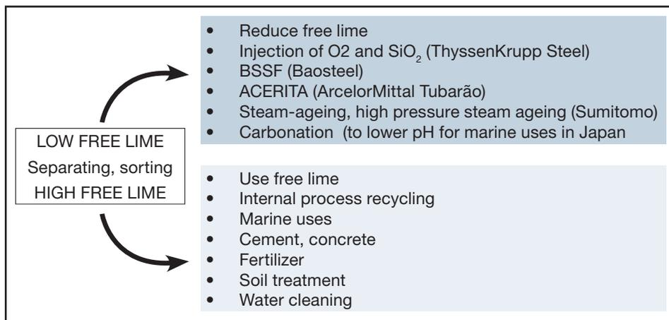
**Figure 31: The two approaches to solving the free lime issue**
