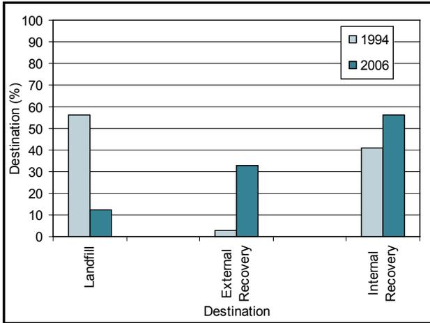
**Figure 73: BOF primary and secondary dust and sludge main destination**
