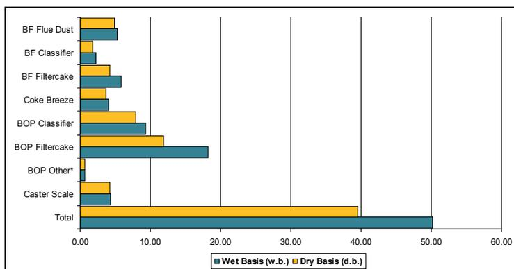
**U.S. Steel Figure 2: Dust, sludge and scale generation at the Edgar Thomson Plant, kg per ton of liquid steel**
