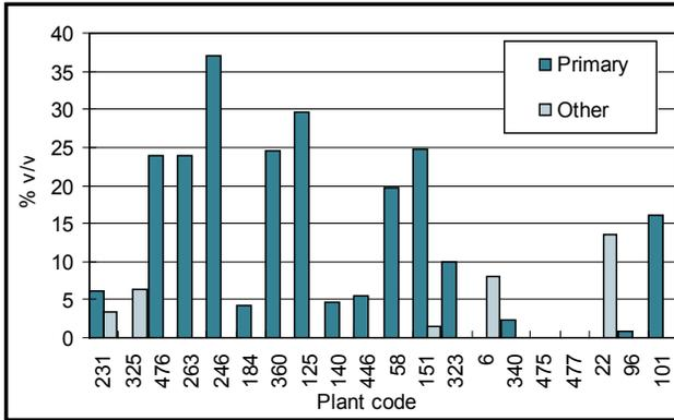
Figure 76: EAF dust and sludge zinc content by plant
