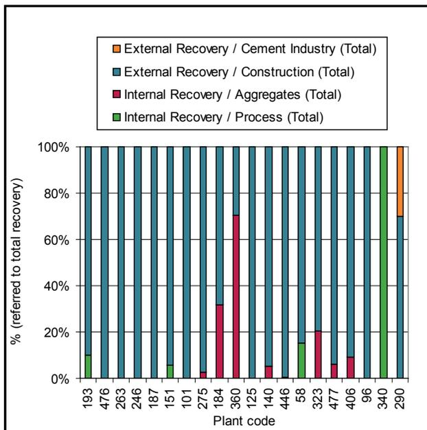
Figure 42: Details of internal and external recovery for EAF slags
