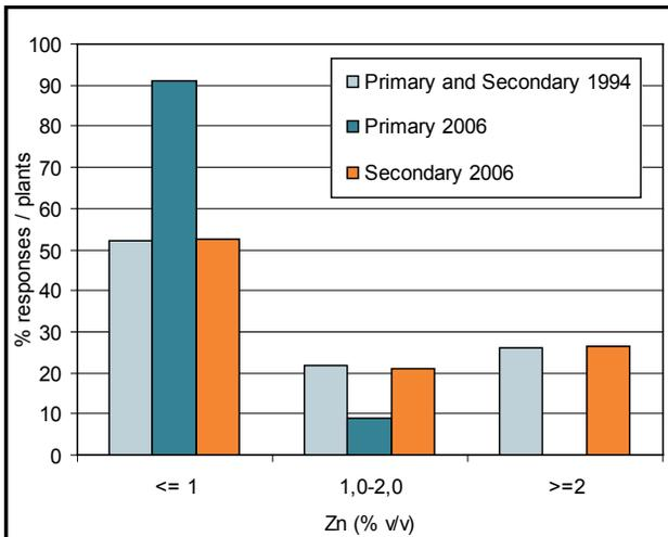
**Figure 71: Comparison of BOF dust and sludge Zn content with 1994 study**
