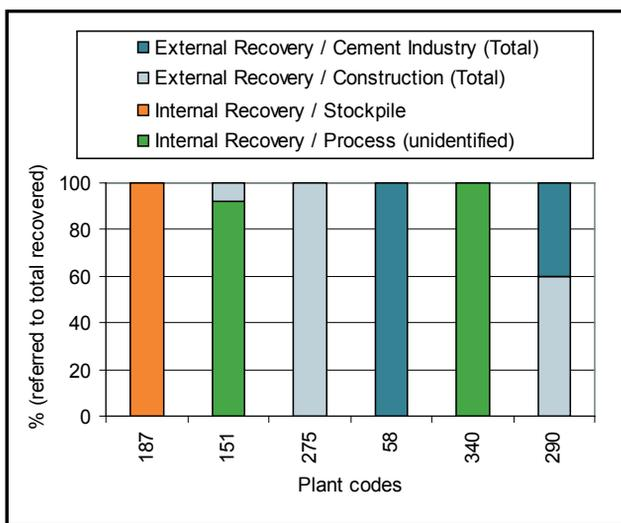
Figure 47: Details of internal and external recovery for EAF SM slags
