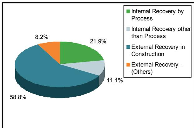
**Figure 24: Main recovery destinations of BOF slag**
