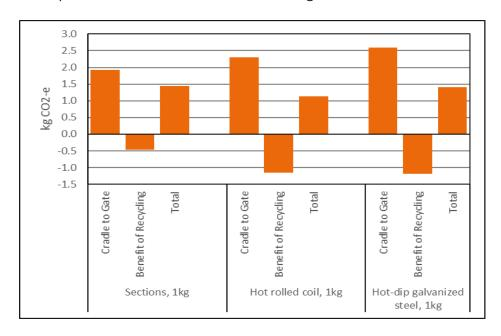
Figure 4: Global warming potential (CO<sub>2</sub>-e) of steel products
