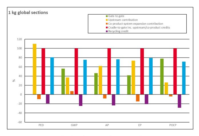
Figure 15: Life cycle contribution to PED and impact categories for sections
