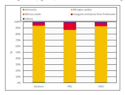
Figure 9: Contributions to eutrophication potential of steel products
