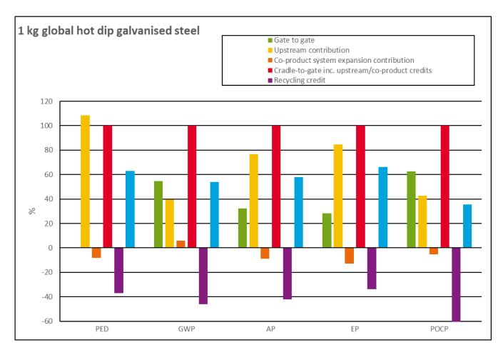
Figure 17 Life cycle contribution to PED and impact categories for HDG
