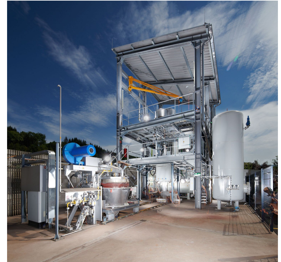
SuSteel pilot plant Direct steelmaking by hydrogen plasma smelting reduction of ultrafine iron ores
