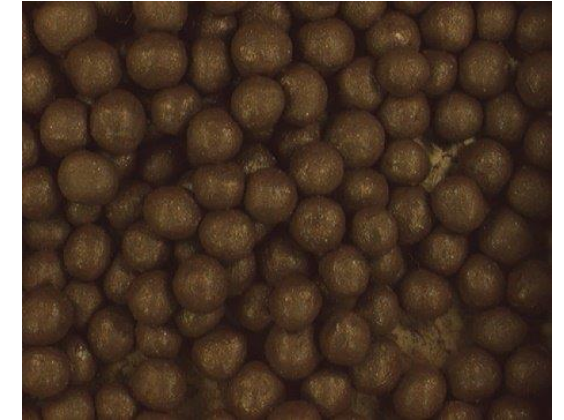
Green Pellets with different binders (bentonite and organic)
