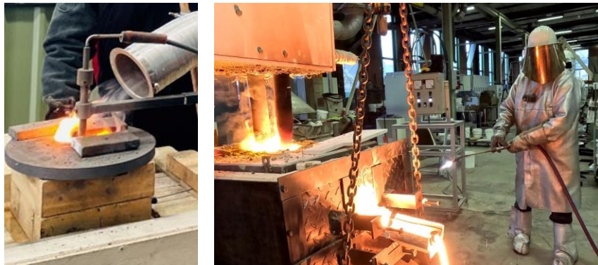
5 kg-scale ESF testing at the University of Newcastle (left). Tapping the 100 kg-scale ESF at University of Duisburg-Essen, Germany (right).
