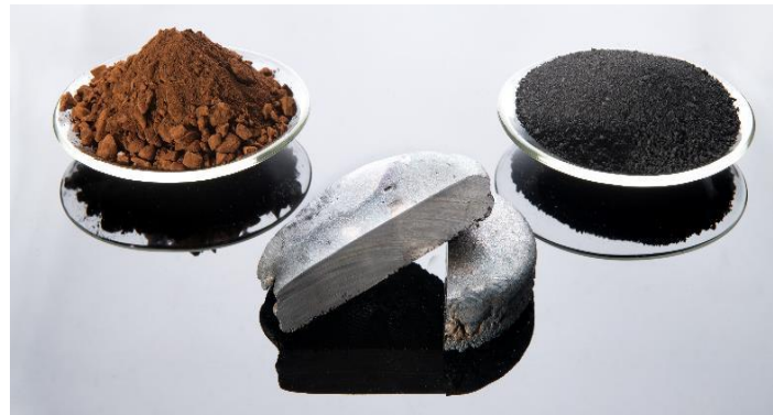
BHP iron ore fines (left), H 2 DRI from BHP fines (right), and iron produced by electric smelting of BHP DRI (centre).
