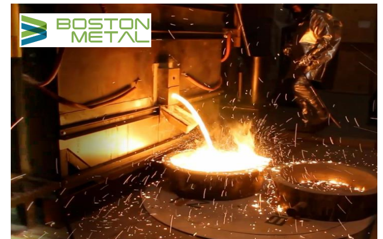
High temperature – Boston Metal MOE metal tapping
