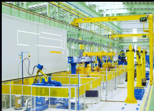
Robotic Welding Workstation for Corbel Joints 牛腿机器人焊接工作站
