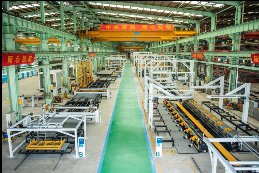
Intelligent production line for steel structure modules 钢结构模块智能生产线
