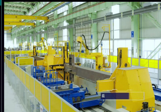
Robotic Welding Workstation for Box Assembly 箱型总成机器人焊接工作站
