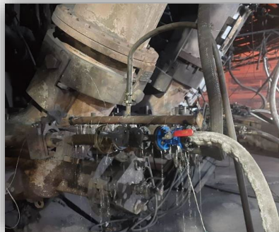
Injection lance set-up through tuyeres
