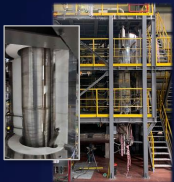
Fluidized Bed Reactor 50 kg/batch
