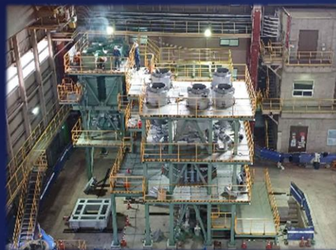
Electric Smelting Furnace 1.0 t/hr (Test will start in 2024)
