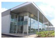
A warehouse built in 2000 in Slough, UK, with a floor space of 3,320m<sup>2</sup> was re-erected in a different location in 2015, using the same steel structure. The savings associated with this project were quantified as follows:
