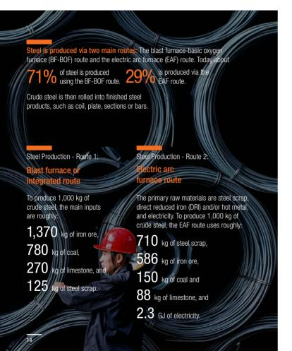
An electric arc furnace can be charged with
