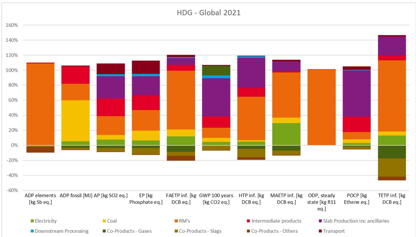
Figure 14: Impacts of steelmaking breakdown - HDG
