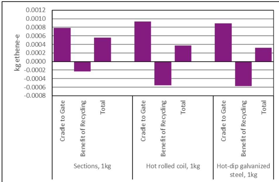
Figure 10: Photochemical ozone creation potential (C<sub>2</sub>H<sub>4</sub>-e) of steel products
