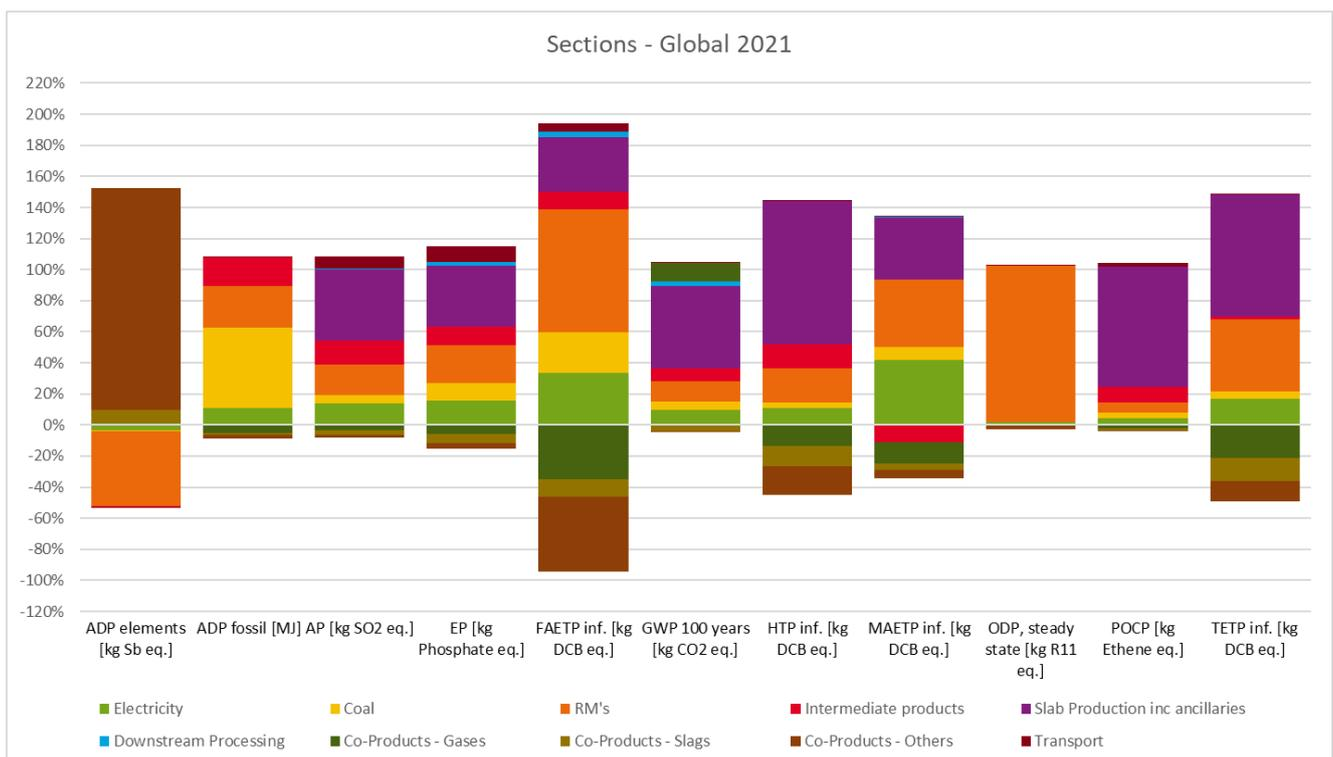
Figure 12: Impacts of steelmaking breakdown - Sections
