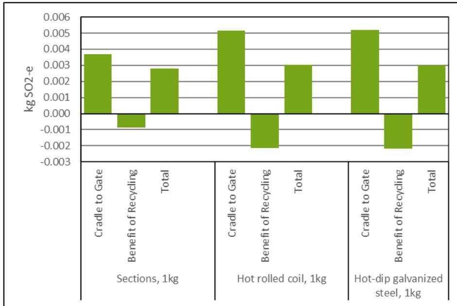
Figure 6: Acidification potential (SO<sub>2</sub>-e) of steel products
