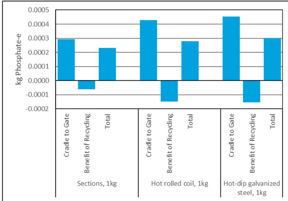
Figure 8: Eutrophication potential ( $PO_4^{3-}$ -e) of steel products
